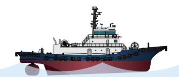
L.O.A : 38.20 m BREADTH : 10.30 m DRAUGHT : 4.5M GROSS TONNAGE : 396 GT MAX.SPEED : 13.00 knots BP, MAX : 64 ton MAIN ENGINES : YANMAR 6EY26W / 2,450PS x 750RPM 2SETS PROPULSION : KONGSBERG US 205 P20 FP 1,802kW x 750 RPM (100% MCR) GENERATOR : 168kW(210KVA) x AC225V x 60Hz x 3PH x 1800RPM ACCOMMODATION : 6 persons FUEL CAPACITY (m<sup>3</sup>) : 81m<sup>3</sup> FRESH WATER CAPACITY (m<sup>3</sup>) : 27.45m<sup>3</sup>
